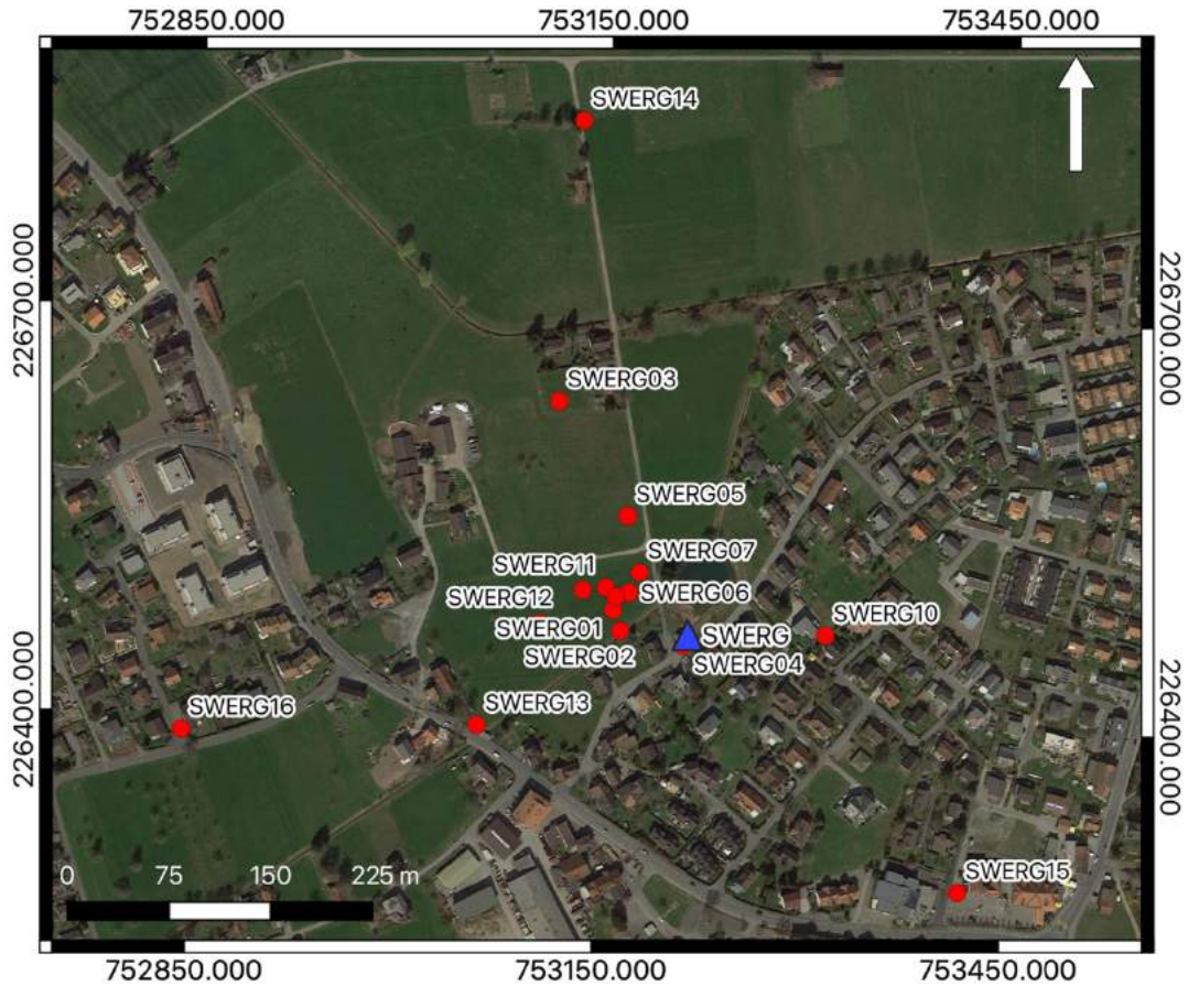
Figure 8: Layout of the array measurement in Werdenberg. The locations of the stations for the passive seismic measurement are indicated by red dots. The blue triangle indicates the seismic station SWERG. Source: Federal Office of Topography.
