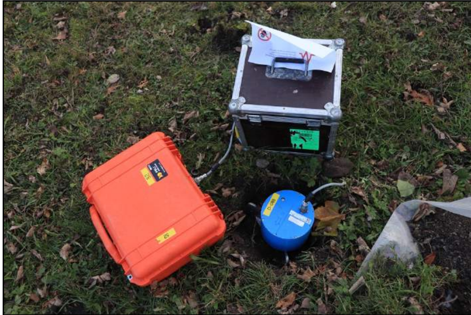
Figure 7: Seismic station installation example for the measurement in Werdenberg.
