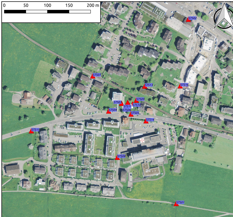
Figure 2: Background topography, strong motion station location and array configuration
