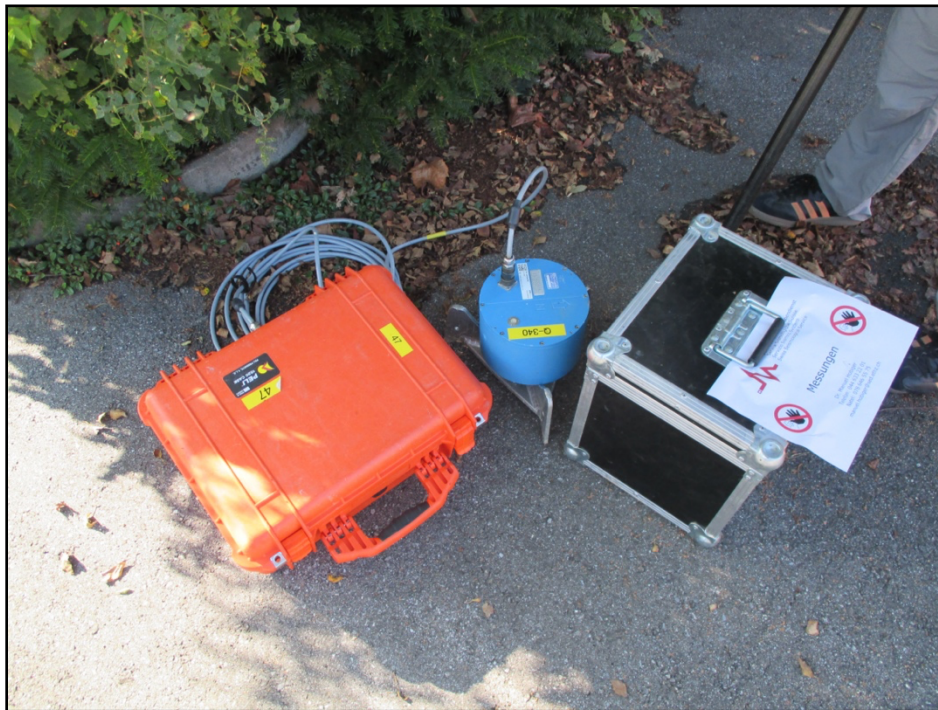
Figure 3: Seismic station installation example for the measurements in Meiringen.
