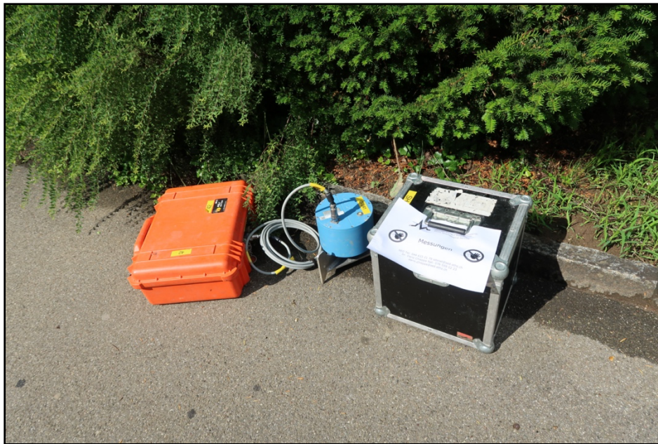
Figure 3: Seismic station installation example for the measurements in Liestal.
