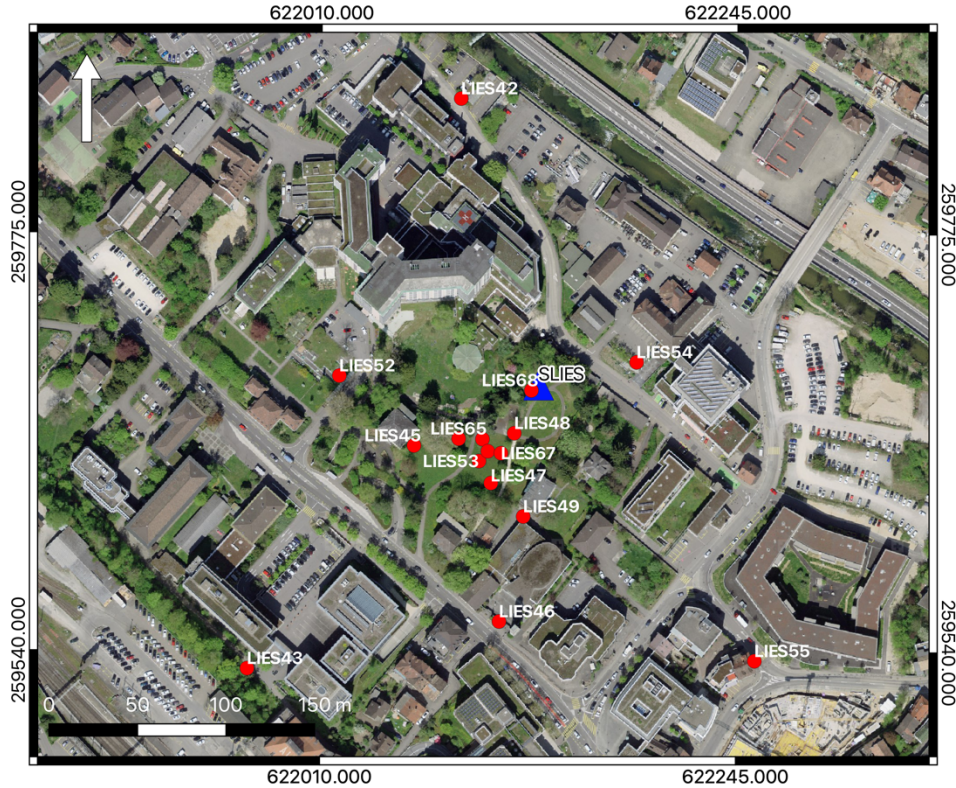
Figure 4: Layout of the array measurement in Liestal. The locations of the stations for the passive seismic measurement are indicated by the red dots. The blue triangle indicates the seismic station site. Source: Federal Office of Topography.
