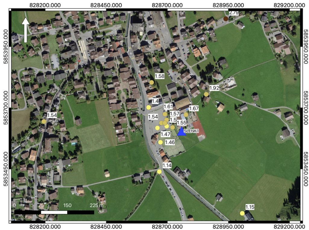
Figure 7: Map showing the variation in frequency for the H/V fundamental peak over the area of Lenk. Source: Federal Office of Topography.
