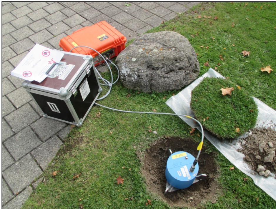
Figure 4: Seismic station installation example for the measurements in Lenk.
