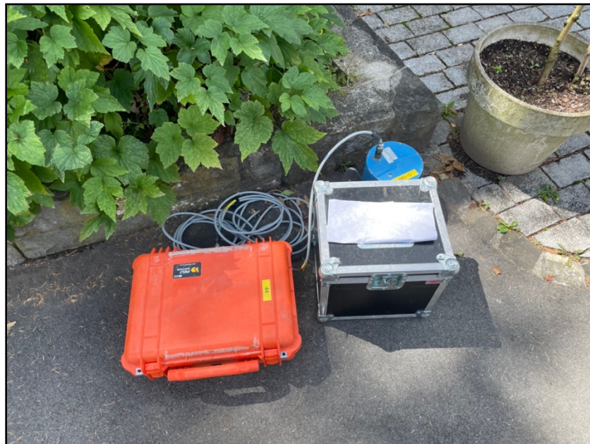
Figure 3: Seismic station installation example for the measurements in Kriens.
