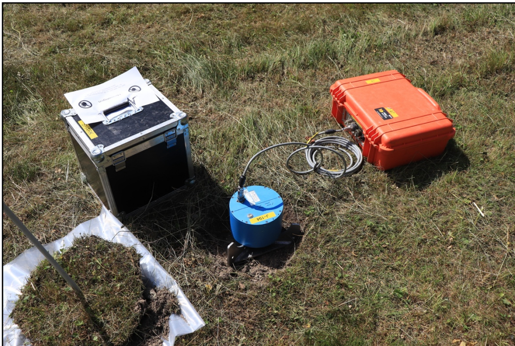
Figure 3: Seismic station installation example for the measurements in Zinal.
