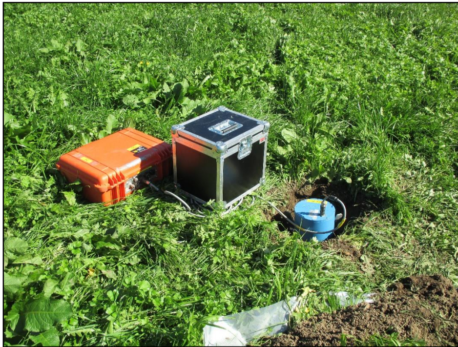
Figure 3: Seismic station installation example for the measurements in Schwyz.
