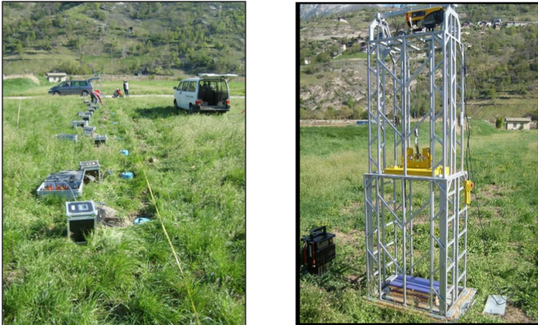
Figure 12 – Visp, MASW survey at SVISP site. Left: recording array in place. Right: Weight-drop source (from Wallimann, 2011).
