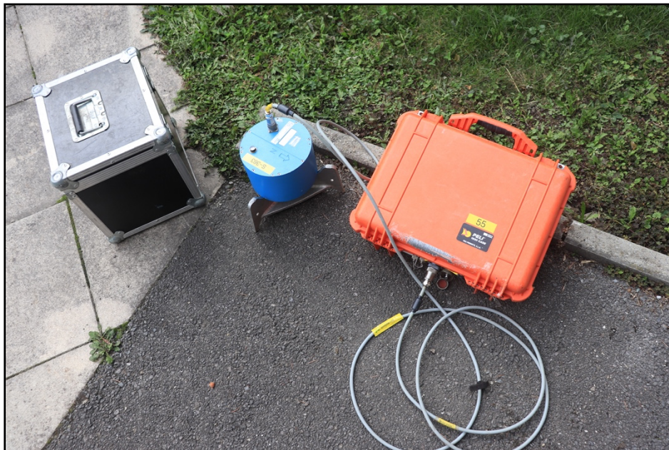
Figure 3: Seismic station installation example for the measurements in Saint-Maurice.
