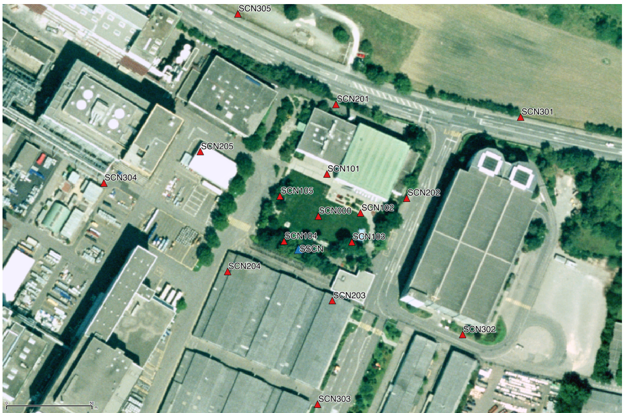
Figure 2: Layout of the array measurements at site SSCN.
