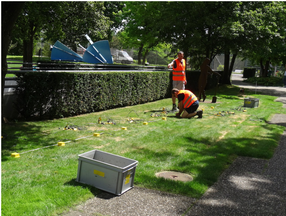
Figure 1: Station SSCN (foreground) during the deployment of the geophone line.
