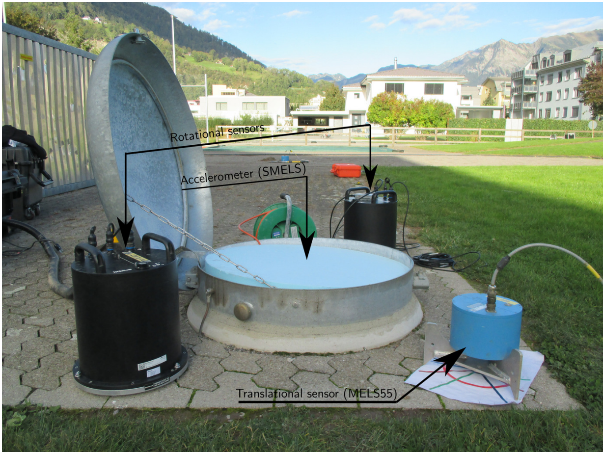
Figure 3: Rotational and translational (MELS55) sensors around the permanent strong motion station (SMELS).
