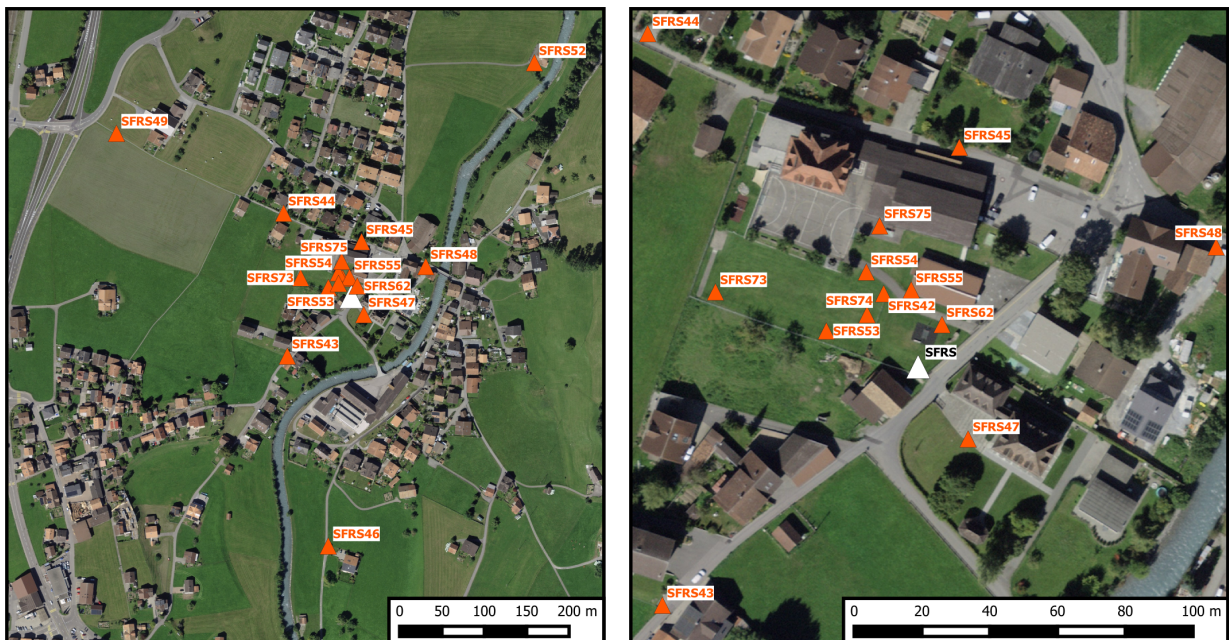
Figure 3: Layout of the array measurements around station SFRS (left) and zoom on the central part of the array (right). The location of SFRS is indicated by the white triangle, the locations of the stations for the passive seismic measurement by the orange triangles. Source: Federal Office of Topography.
