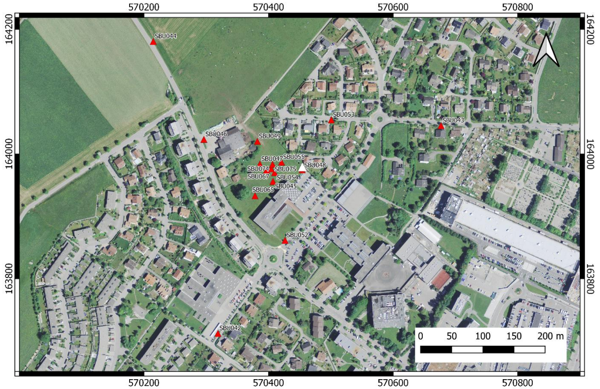
Figure 4: Layout of the array measurement in Bullé. The locations of the stations for the passive seismic measurement are indicated by the red triangles. The white rectangle indicates the seismic station. © 2020 swisstopo (JD100042)
