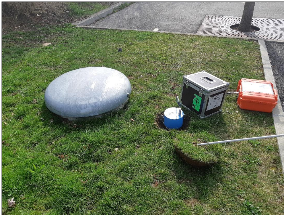
Figure 3: Seismic station installation example for the measurements in Bulle.
