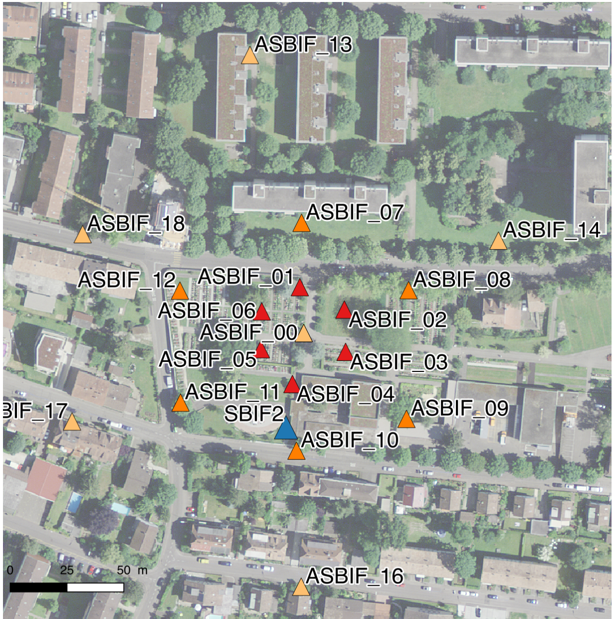
Figure 4: Layout of the array measurements at site SBIF2. The array stations from the different configurations are in red to light orange and station SBIF2 in blue.
