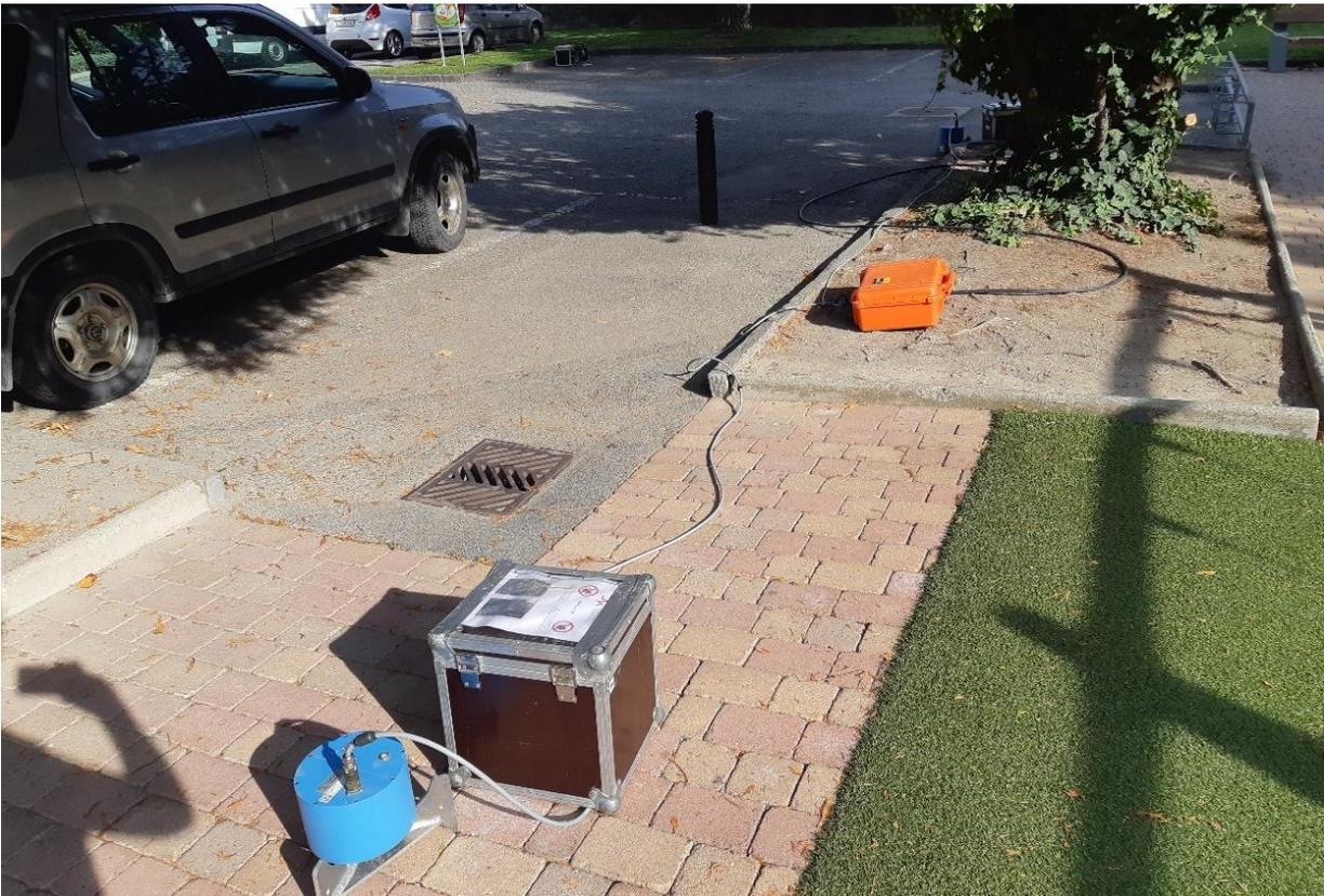
*Figure 4: Seismic station installation example for the measurement in Ardon.*
