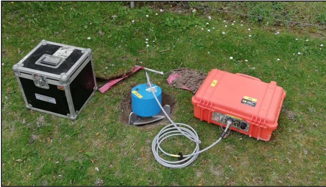
Figure 3: Seismic station installation example for the measurements in Aarau.
