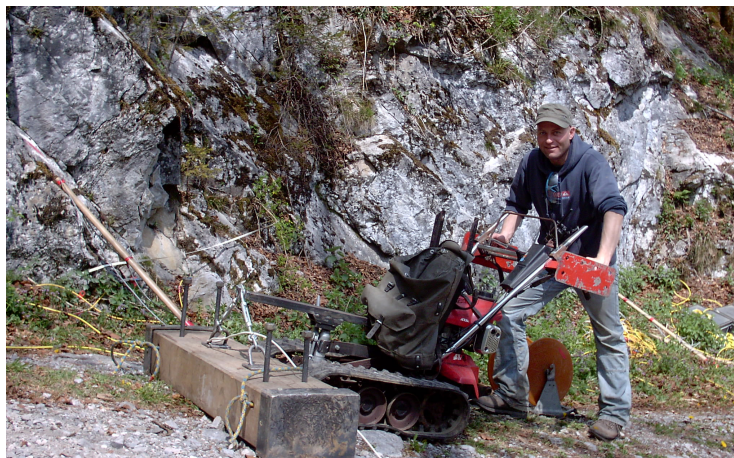
Fig. 2.1: S-wave data acquisition at profile 09SN_20WIMIS-S2 with a small motorized wheel barrow to transport the shear wave generator to the site in difficult areas.
