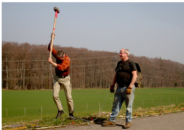
Fig. 2.1: P-wave data acquisition at profile 09SN_17TORNY-P1.
