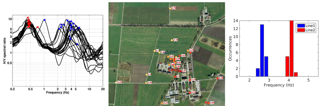
Figure 25: Left: H/V curves from passive array measurements (black lines), with fundamental (red crosses) and secondary peaks (blue crosses). Center: map of the geographical distribution of the secondary peak frequencies. Right: theoretical resonance frequencies corresponding to the clay/turf–sand interface obtained from the best-performing velocity profiles from Fig. 24.
