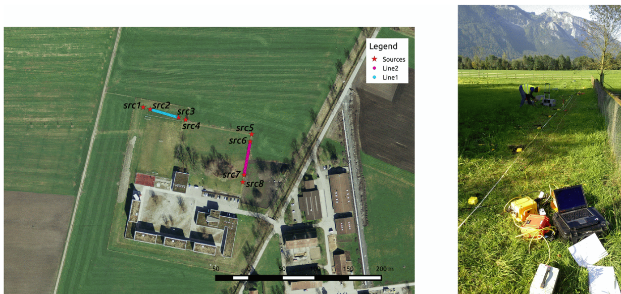
Figure 16: Left: overview map of the active seismic surveys. Right: photo showing the deployment at line 2.
