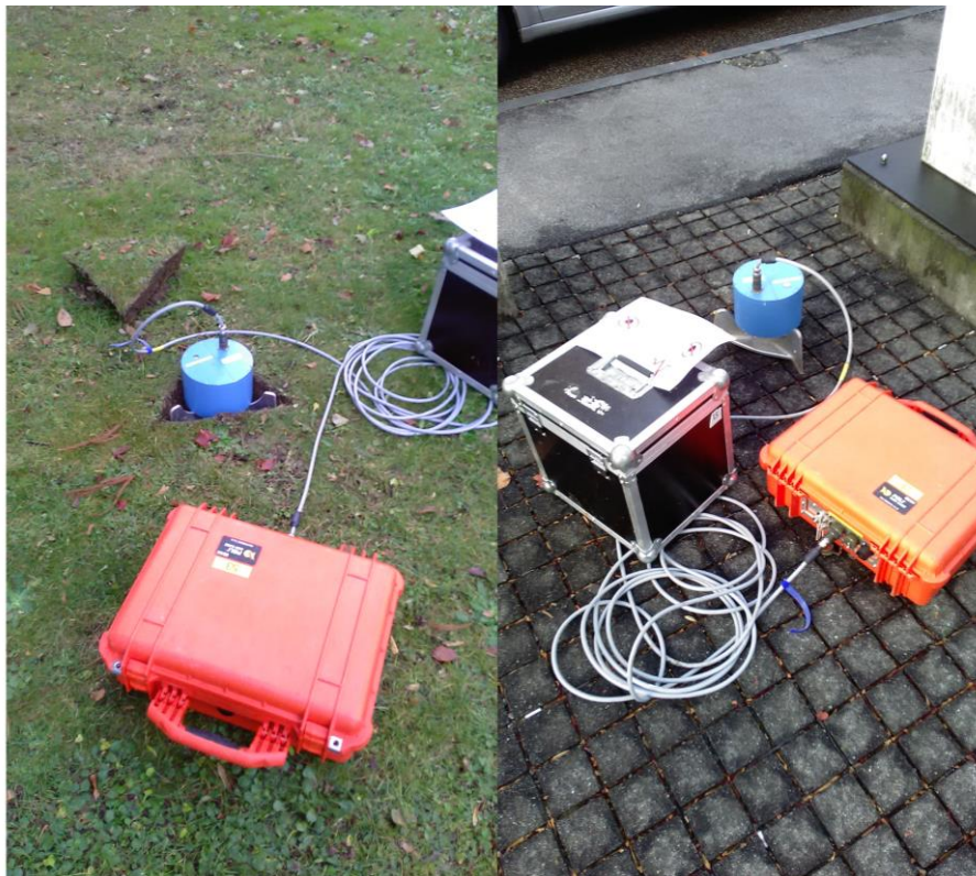
Figure 4 – Examples of station installation. Left: the tripod and the sensor are housed into a small hole dug into the soil. Right: the tripod is directly placed on cobbles.
