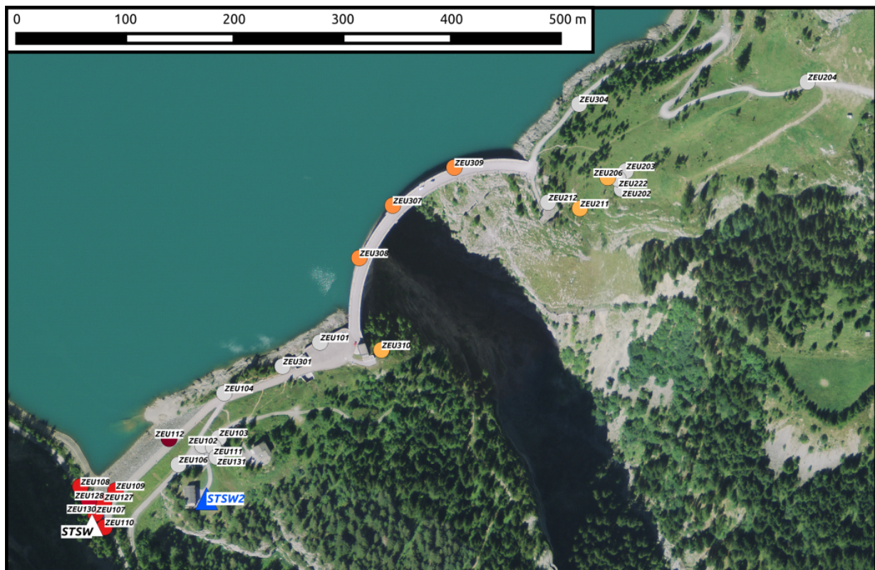
Figure 12: Map with the locations of the H/V measurements. Colored points correspond to points with a visible resonance frequency in the H/V curve, grey points have mainly flat H/V curves. The H/V curves for the different stations are shown in Figs 13-16.
