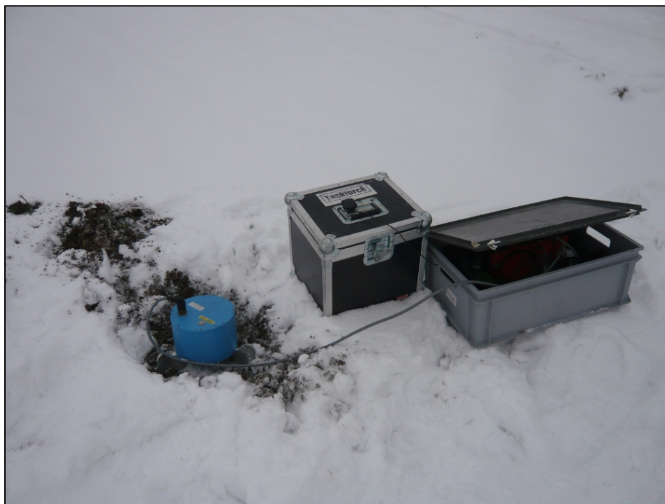
Figure 3 - Single acquisition point of the array, consisting in a Q330 datalogger (gray box on the right) and a Lennartz 5s velocity seismometer (blue, on the left). The coupling of the sensor is assured by removing the uppermost part of the frozen soil and by means of a special support (Trihedron).
