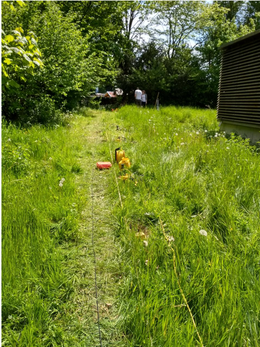
Figure 4 – Geophone array in place. The picture was taken near the north end of the line.
