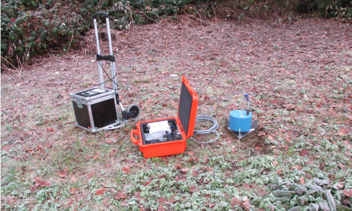
Figure 12 – Single-station ambient vibration recording performed in December 2016.
