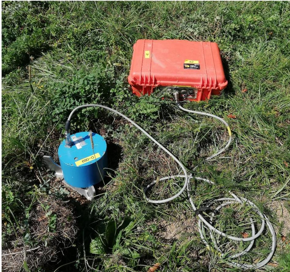
*Figure 7 – Single-station ambient vibration recording ONU008 performed nearby the center of the linear deployment for MASW.*
