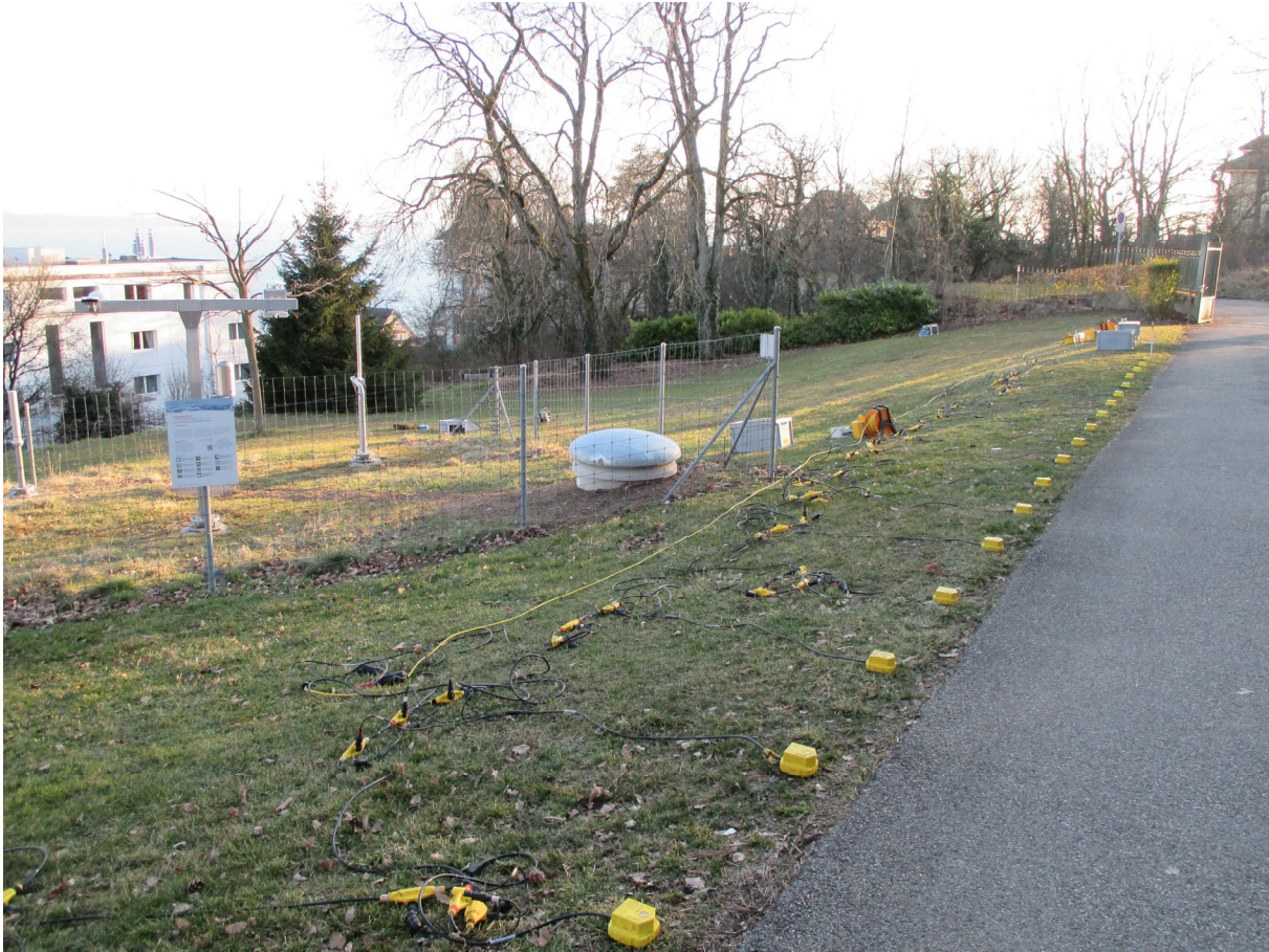
Figure 7 – Deployed geophone spread. Beyond the fence on the left is the vault covering station SNES2.
