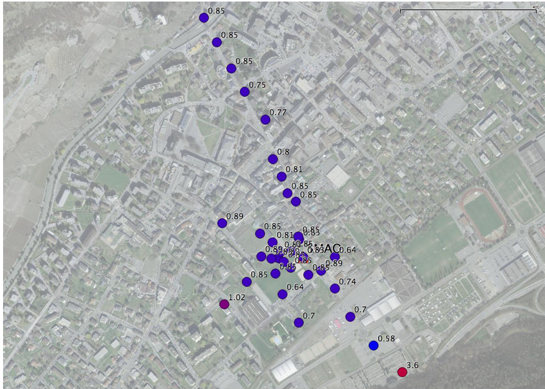
Figure 8: Map of the resonance frequencies (in Hz) in the city of Martigny.
