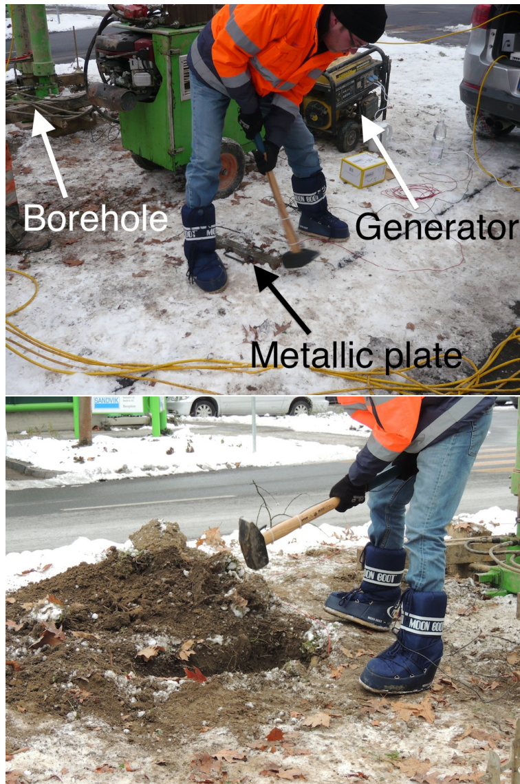
Figure 3: Hammering during the downhole seismic test.
