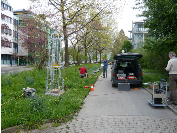
Figure 2: The 120kg dropping mass device which has been used as artificial source to stimulate the generation of Rayleigh waves.
