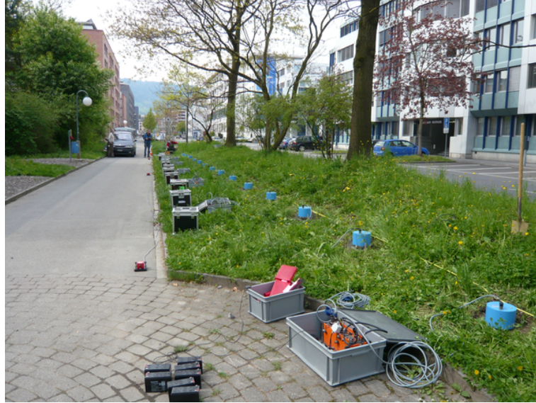
Figure 4: The surface-wave survey line. In the picture, only the 14 high-resolution three-component seismological stations are visible, while the geophone string of 24 elements is hidden in the grass.
