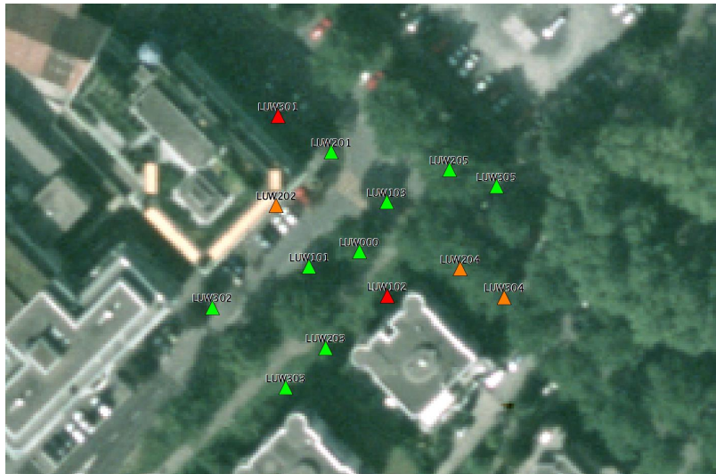
Figure 5: Geometry of the passive array measurement. Color is related to the positioning accuracy obtained on the field after the second measurement. Green: lower than 5 cm, Orange: between 1 and 1.5 m. Red: greater than 1.5 m.
