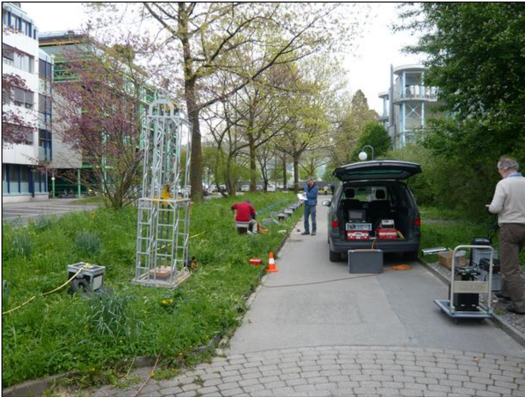
Figure 3. The 120kg dropping mass device which has been used as artificial source to stimulate the generation of Rayleigh waves.
