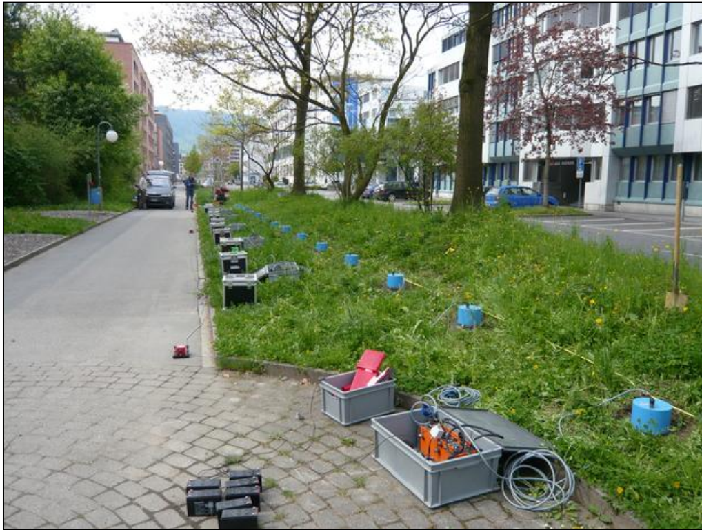
Figure 2. The surface-wave survey line. In the picture, only the 12 high-resolution three-component seismological stations are visible, while the geophone string of 24 elements is hidden in the grass.
