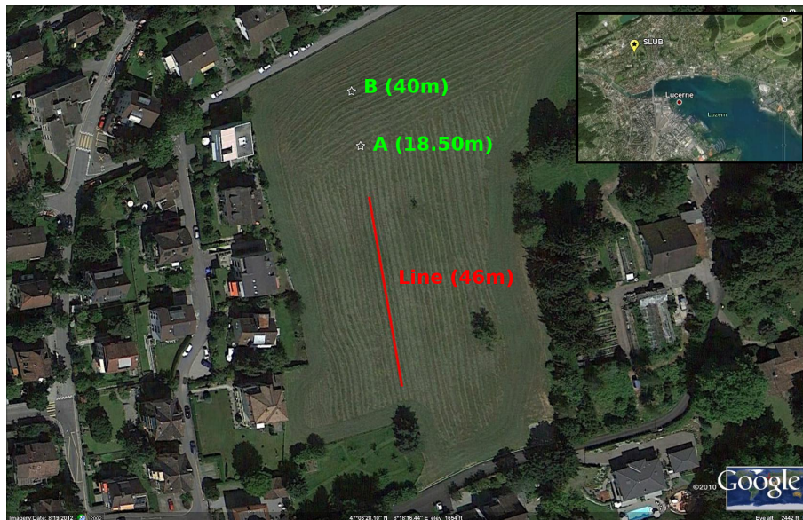
Figure 4: Location of the seismic line (in red) and the two wave-field excitations (A at 18.5 m and B at \approx 40 m) with green stars.
