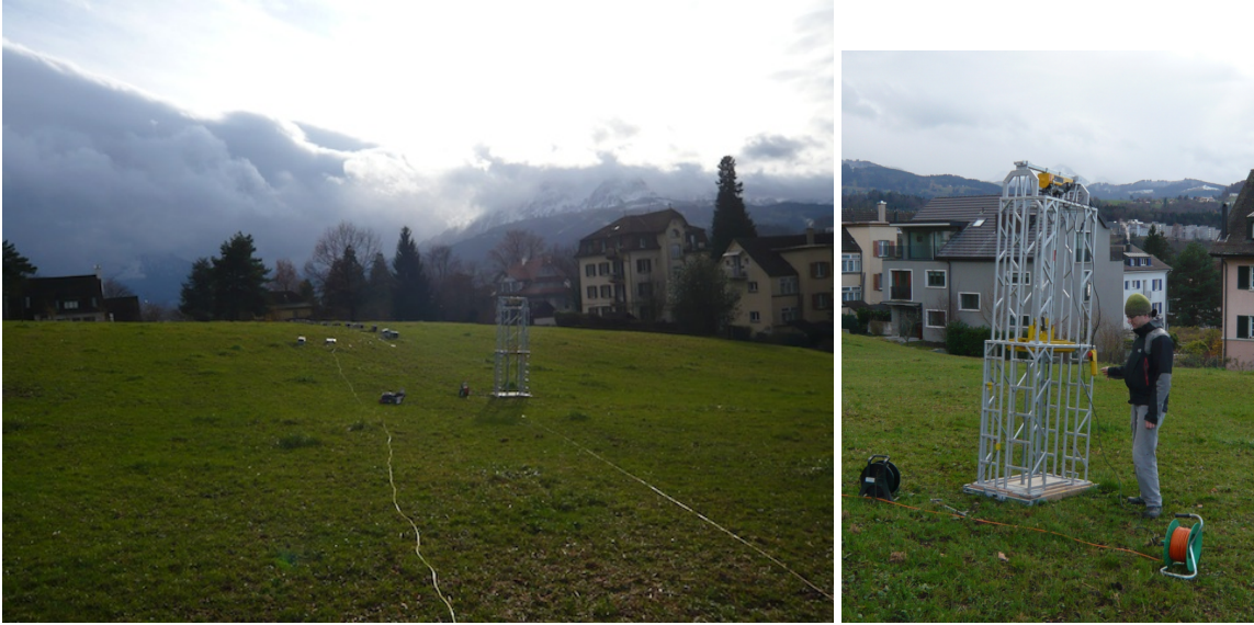
Figure 2: The 120kg dropping mass device which has been used as artificial source to stimulate the generation of Rayleigh waves.
