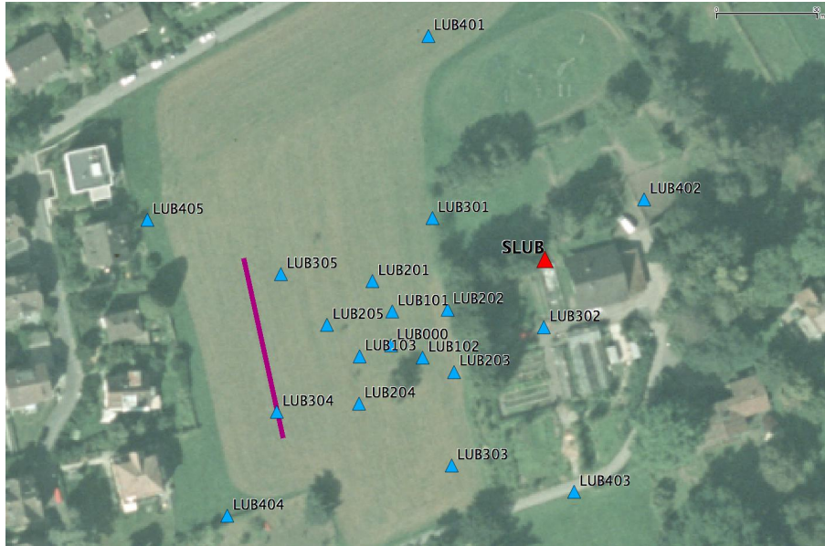
Figure 5: Geometry of the arrays (blue triangles) compared to the seismic line (purple).
