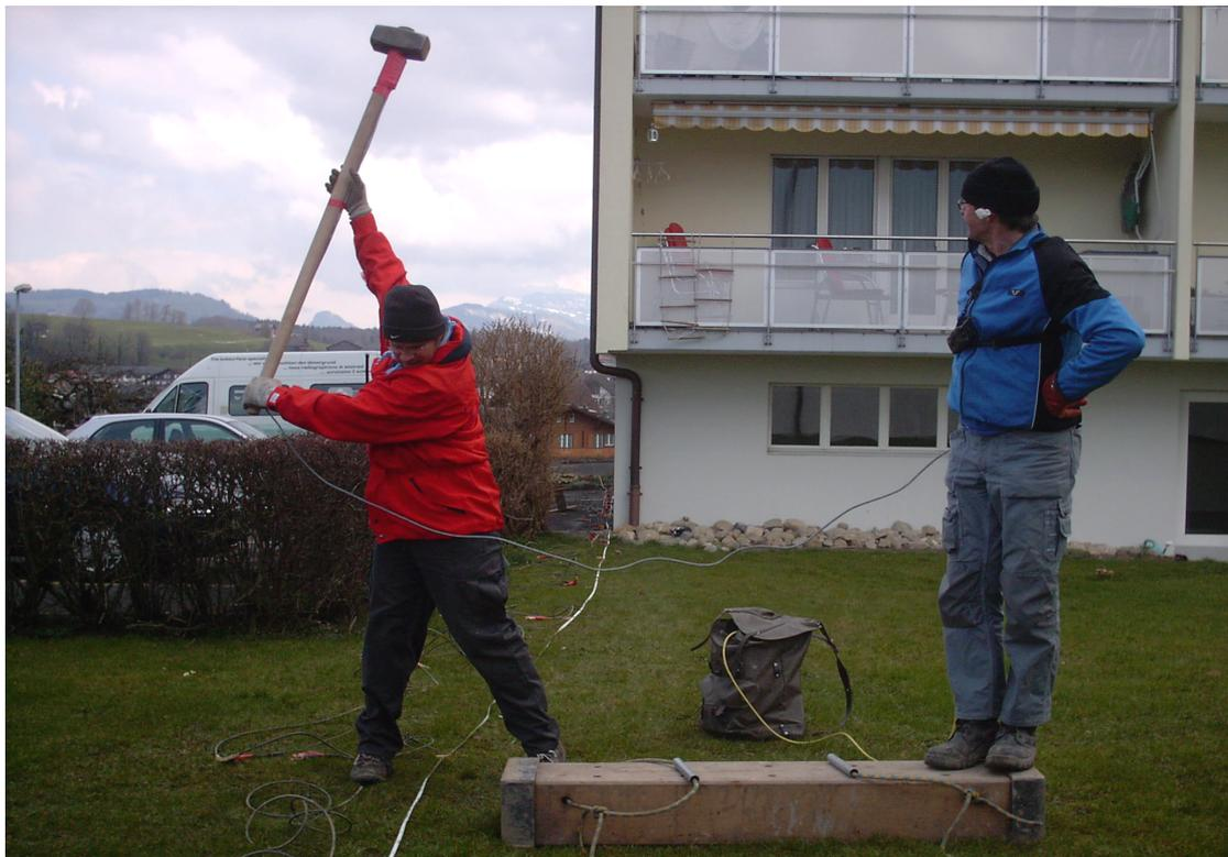
Fig. 2.2: Seismic shear wave data acquisition: striking the metal-plated wooden beam with a 8 kg hammer in both directions (from left and right).
