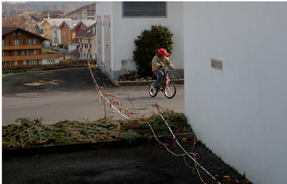
Fig. 2.1: Seismic data acquisition: lay-out of geophone and jumper cables along the house wall. The seismic monitoring station is located in a chamber below the bicycle kid.
