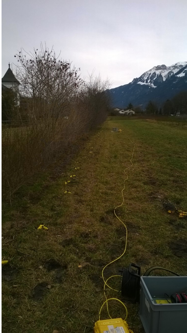
Figure A2 – Seismic array in place.
