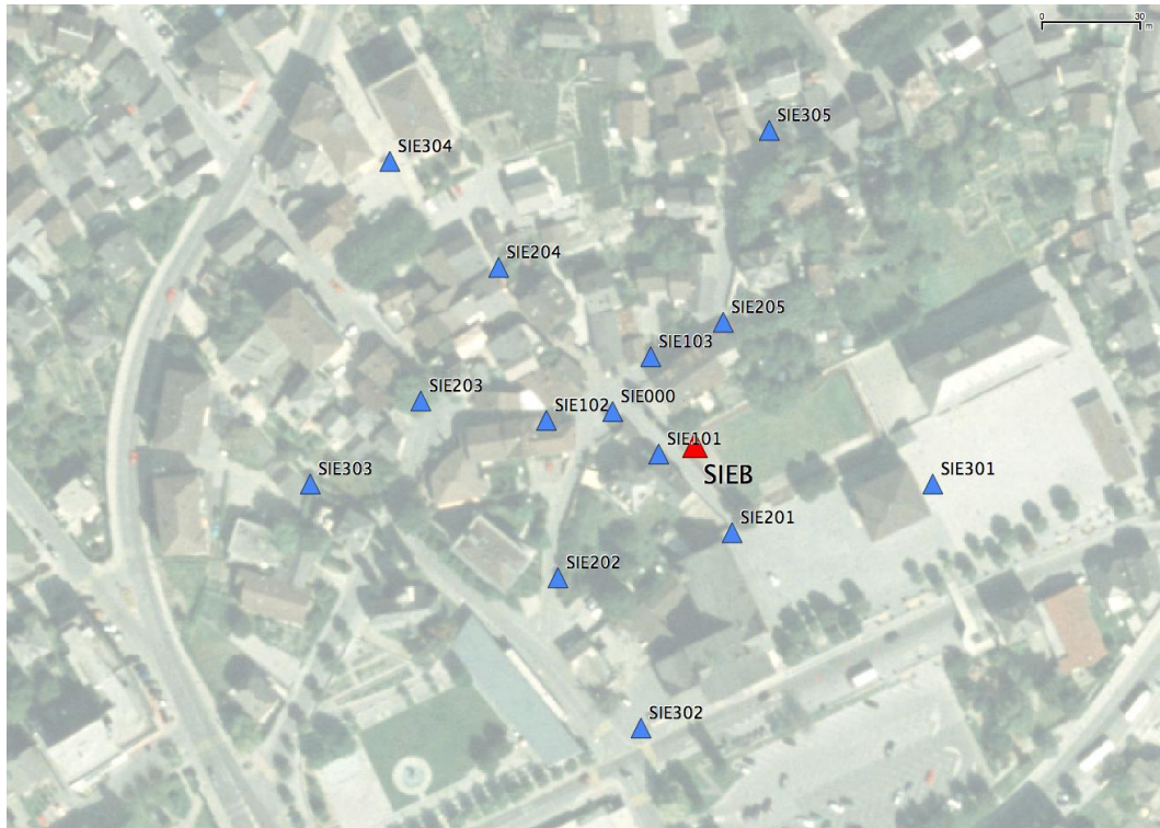
Figure 2: Geometry of the arrays.
