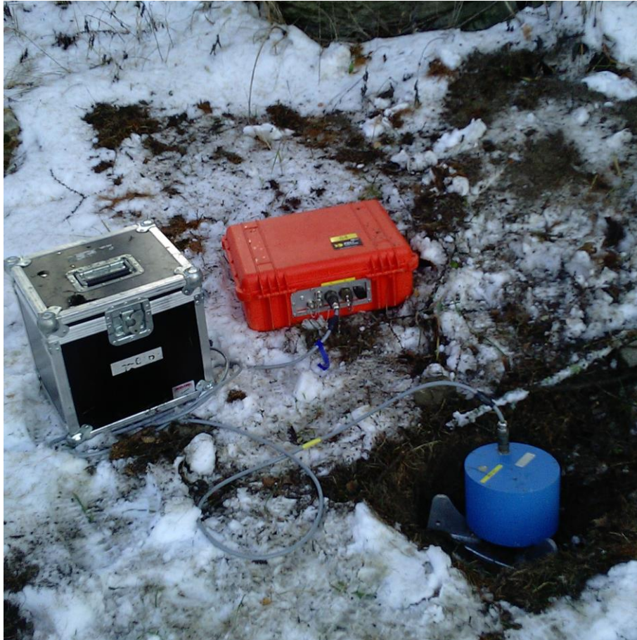
Figure 10 – Deployment of the Lennartz seismometer for microtremor recording.
