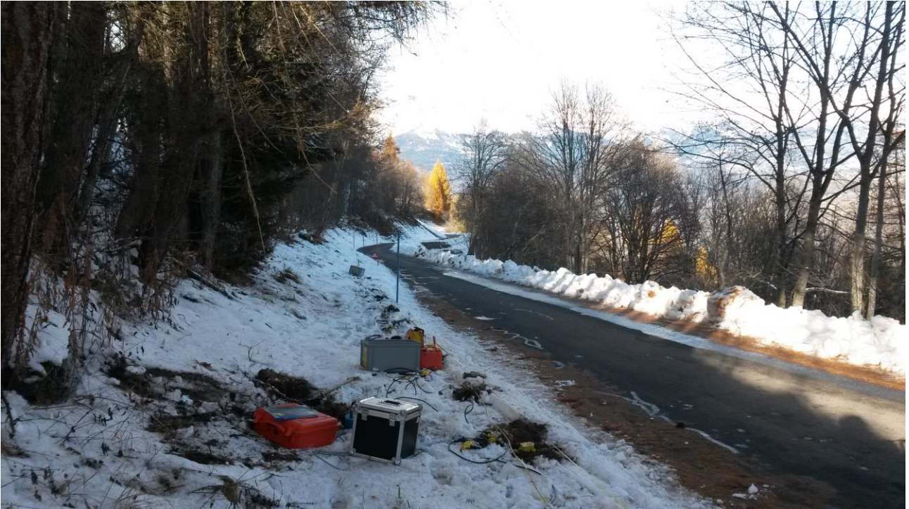
Figure 4 – Geophone array in place. The picture was taken at the south end of the line.
