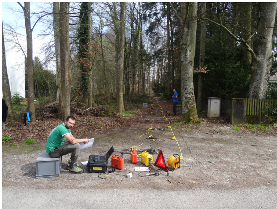
Figure 15: Map representing the location of the active seismic array and of the station SFRU (top: image produced with Google Earth) and picture of the deployment of the seismic array (bottom).
