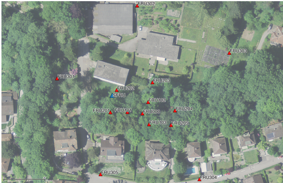
Figure 3: Layout of the passive array measurements at site SFRU. Array stations are in red and SFRU station in blue.
