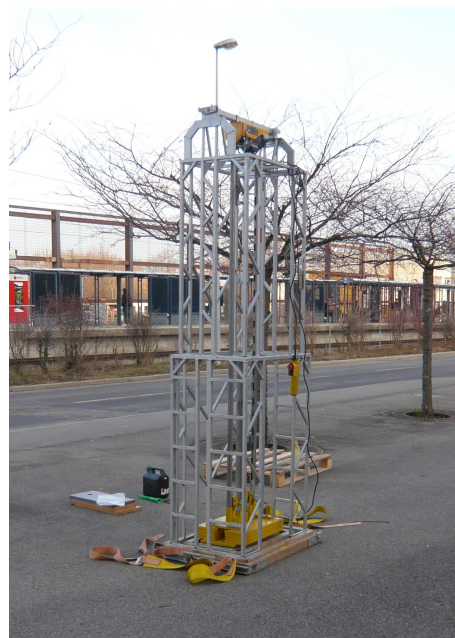
Figure 2: The 120kg dropping mass device which has been used as artificial source to stimulate the generation of Rayleigh waves.
