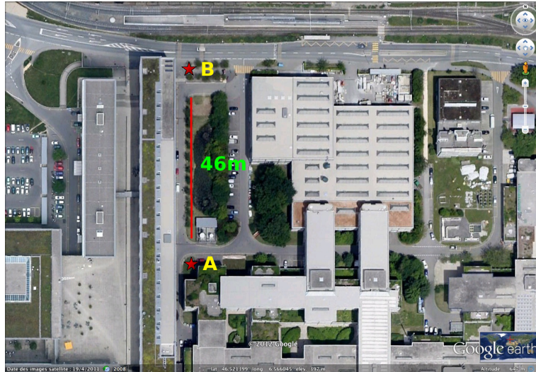
Figure 3: Location of the seismic line (in red) and of the two source locations A and B (red stars).
