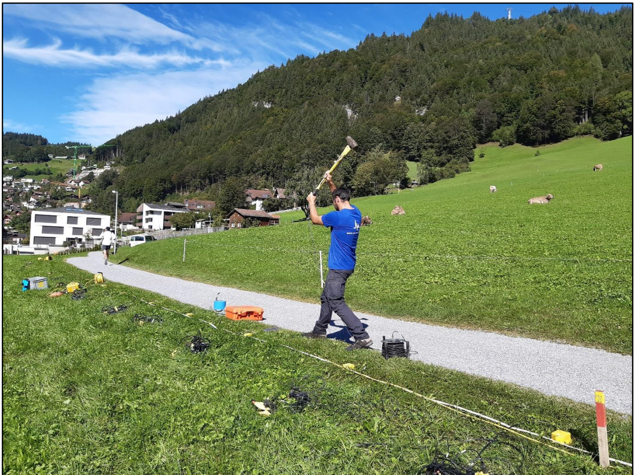
Figure 4: Geophone array in place with example of sledgehammer vertically blown. The picture was taken near the center of the line (view point ESE to WNW).
