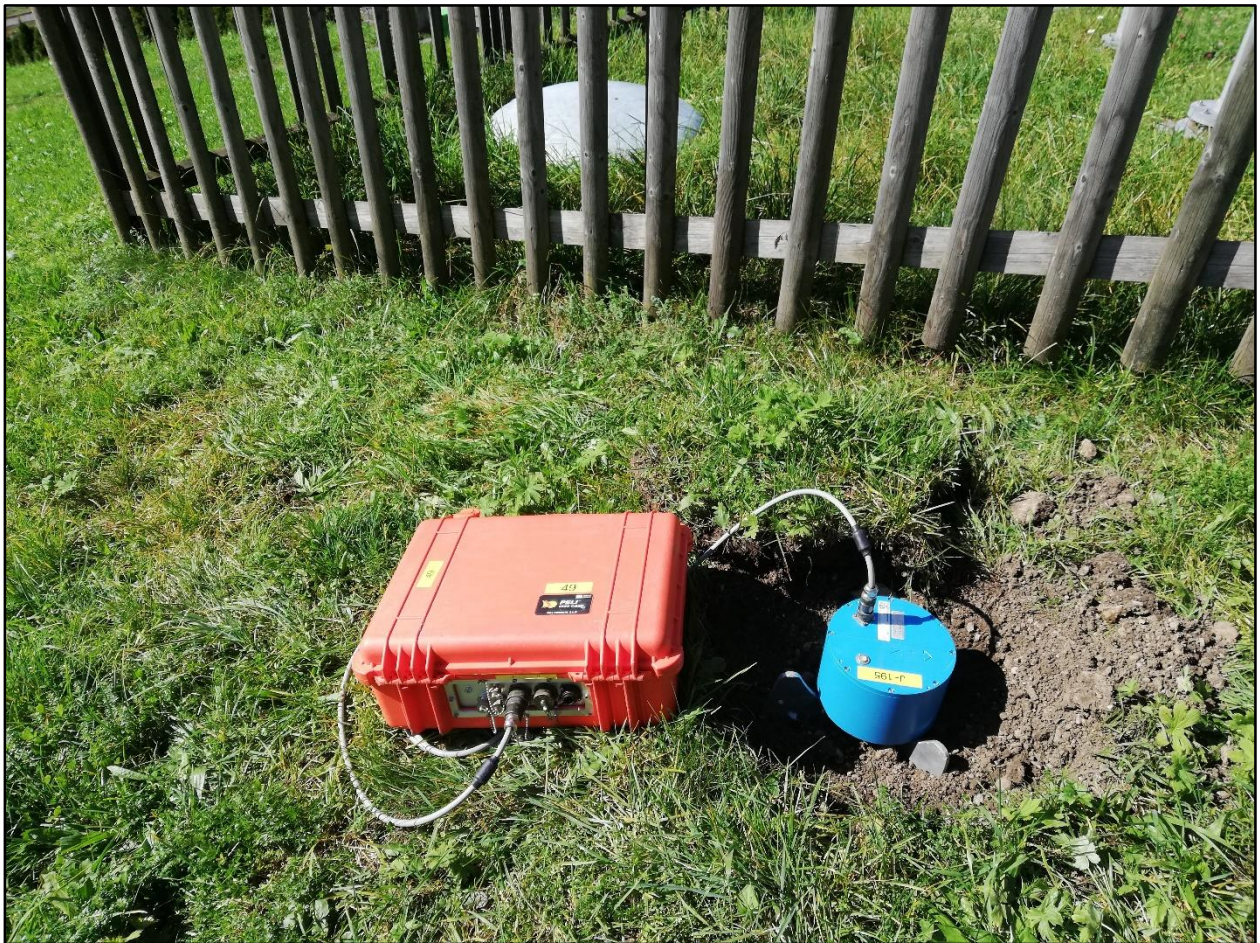
Figure 12 – Single-station ambient vibration recording performed nearby the SENGL seismic station.
