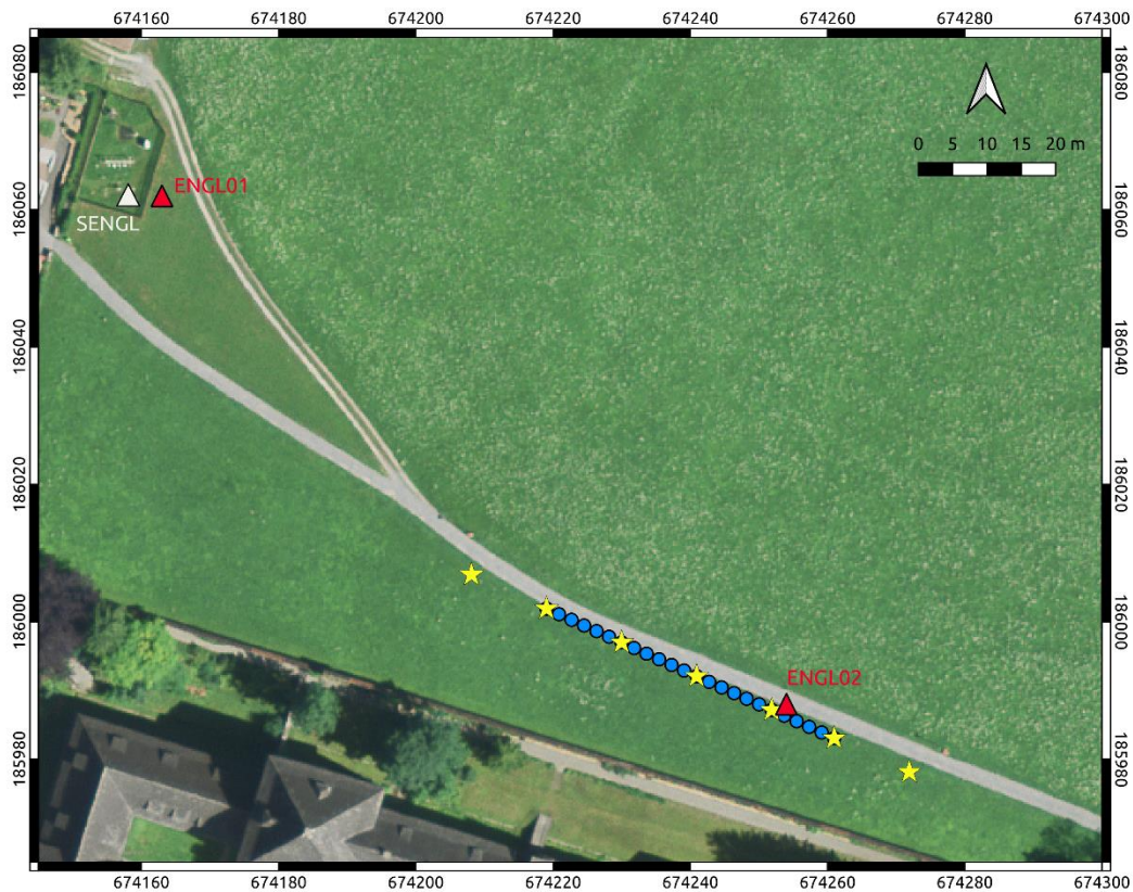
Figure 3: Map representing the position of the targeted station (SEGL, white triangle), of the active seismic line (yellow stars – sources, blue circles - geophones) and of the noise recording sensors (reds triangles).
