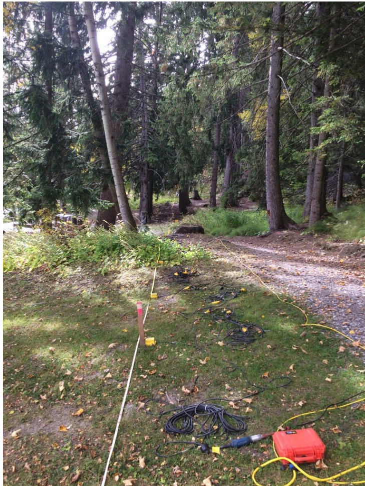
Figure 4 – Geophone array in place. The picture was taken at the north-east end of the geophone line.
