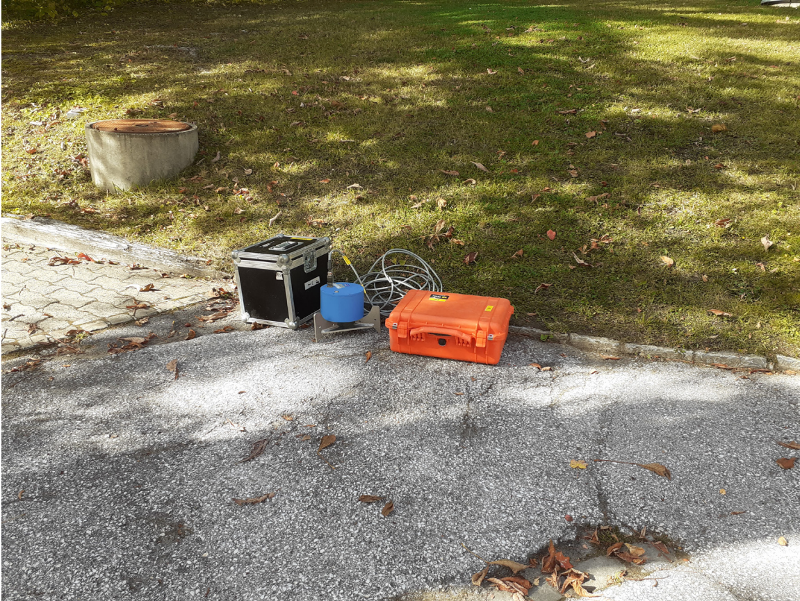
Figure 9 – Deployment of the Lennartz seismometer for microtremor recording.
