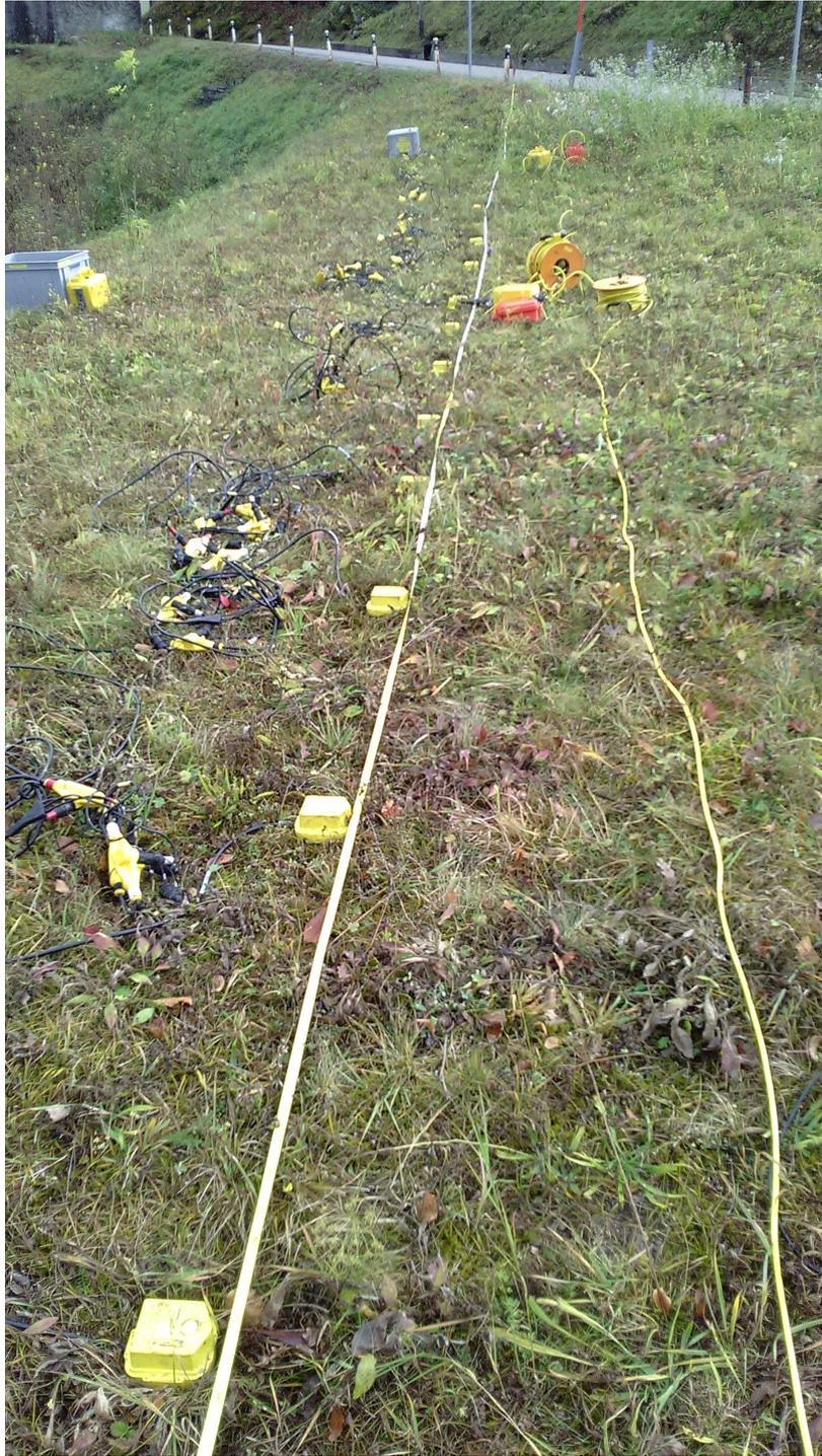
*Figure 4 – Geophone array in place.*
