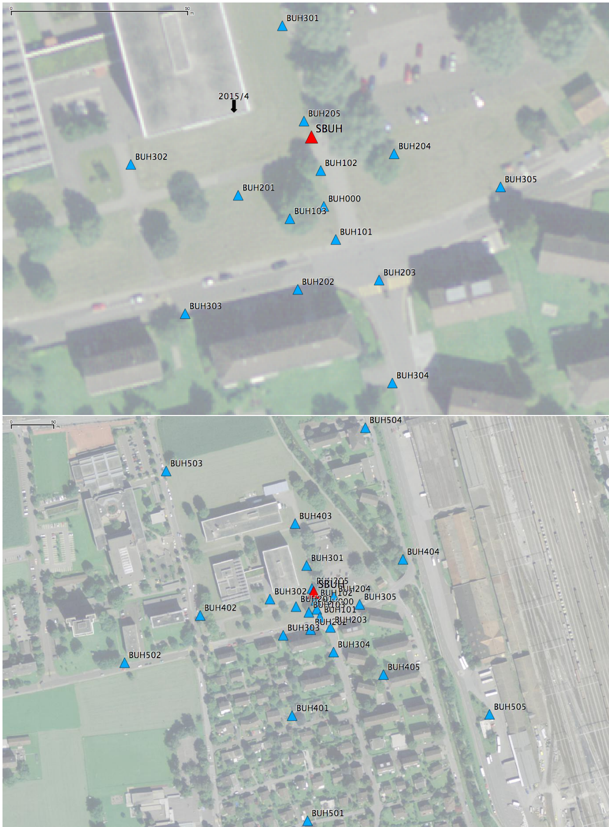
Figure 3: Geometry of the arrays: zoom on the first configuration, including the borehole 2015/4 presented on Fig. 2 (top) and view of the whole experiment (bottom).
