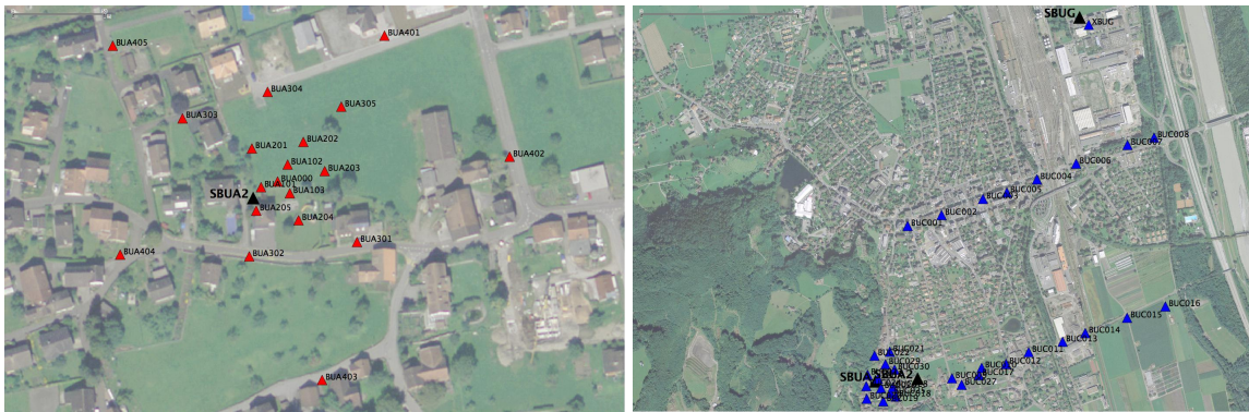
Figure 2: Geometry of the arrays of the first campaign (left) and single points recorded during the second campaign (right).
