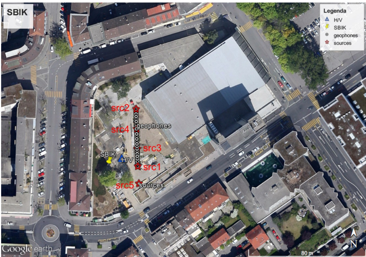
Figure 3 – Map representing the position of the targeted station (SBIK), of the active seismic line and of the noise recording sensor (labelled H/V; © 2016 GoogleMaps).
