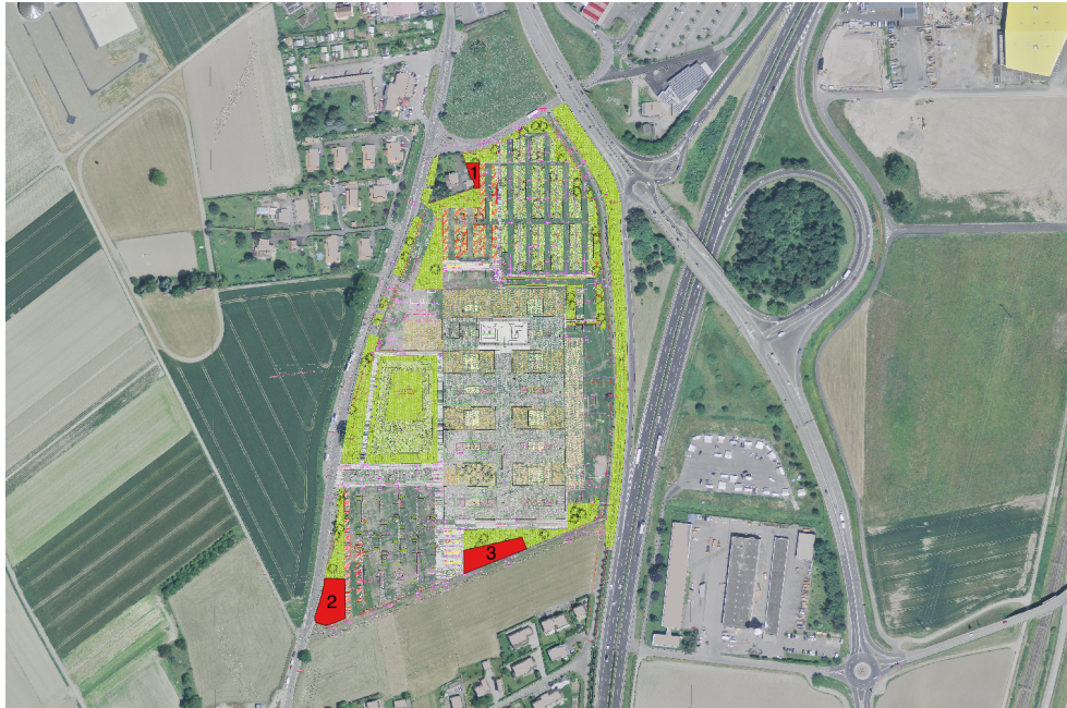
Figure 1: Hospital project superimposed on the aerial view of the area. Red zones correspond to pre-selected zones for a possible installation of the seismic station (orthophoto: © 2016 swisstopo JD100042).
