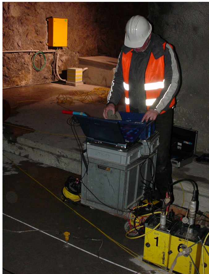
Fig. 2.3: Improvisational seismic data registration in the gallery at SED station LLS. The yellow boxes in the foreground contains 24 channel A/D converter each. The sensors (yellow case in the middle foreground) are firmly plugged in small holes drilled into the concrete foundation of the gallery's bottom. In the background the cabinets with the earthquake monitoring station instrumentation.
