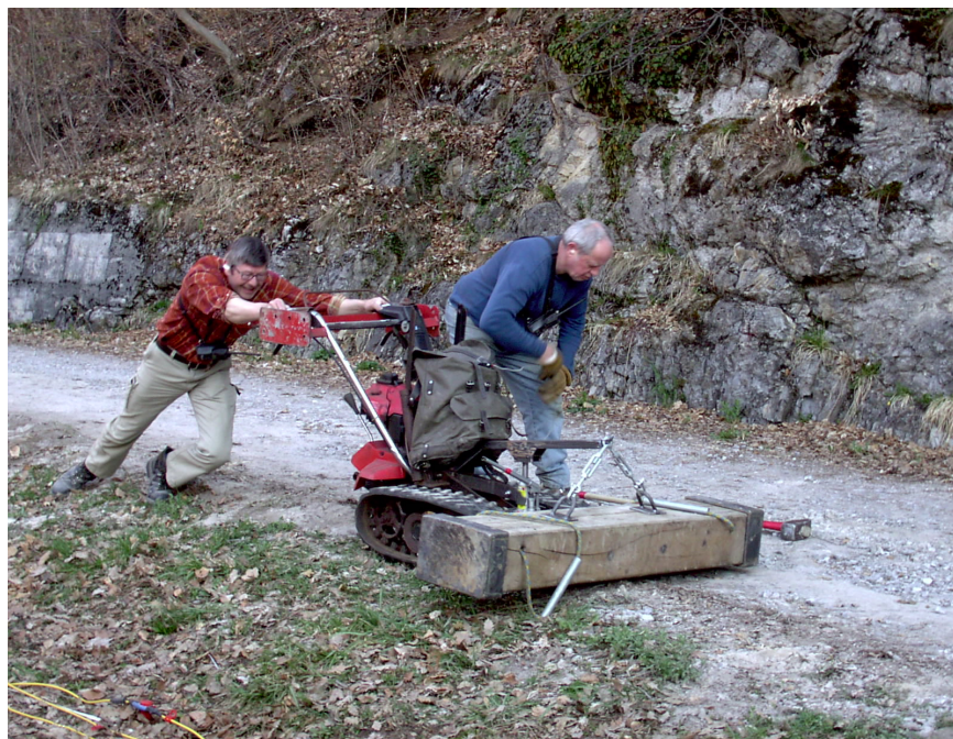
Fig. 2.5: S-wave source transportation along the seismic profile at SED station AIGLE.
