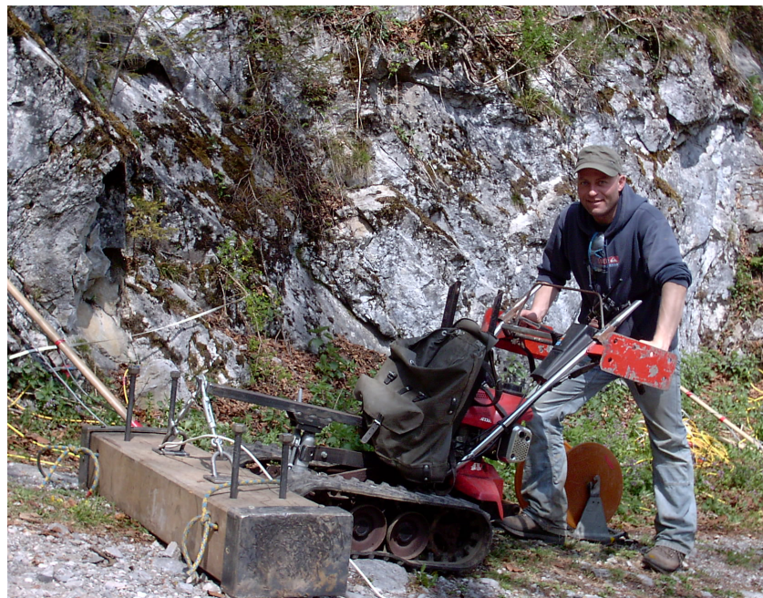
Fig. 2.1: S-wave data acquisition at SED station WIMIS. In front of the motorized wheel-barrow the seismic shear wave source with steely spikes for fixation at ground.
