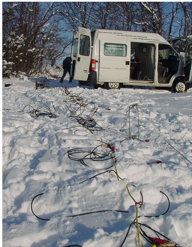
Fig. 2.6: Geophone lay-out and monitoring car at SED station SULZ.
