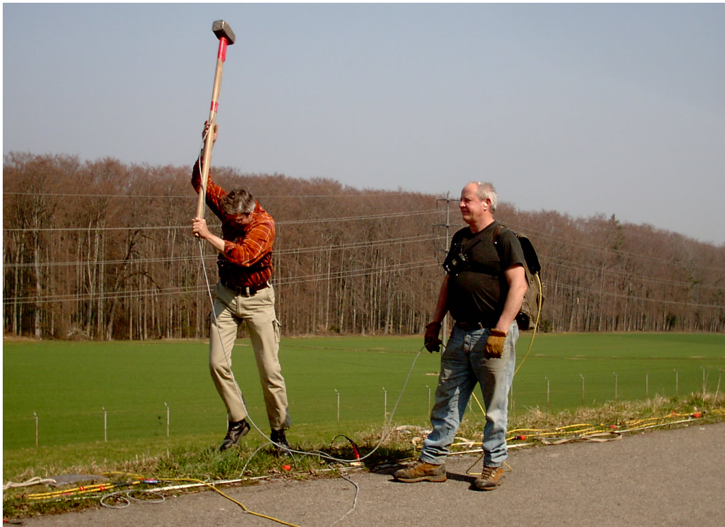
Fig. 2.2: Man-powered p-wave data acquisition at SED station TORNY striking the metal plate (left in the pasture) with the 8 kg hammer. The backpack contains the radio link for trigger signal.
