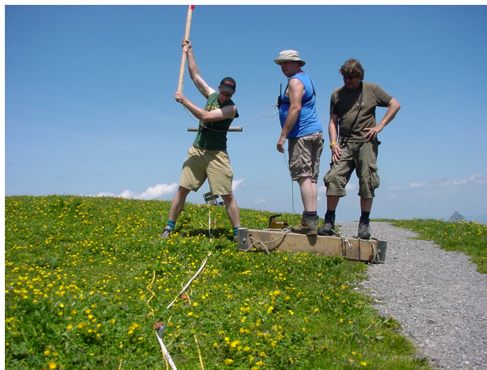
Fig. 2.1: S-wave data acquisition at profile 09SN_11MUO-S1.
