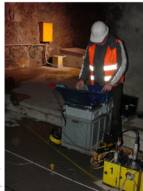
Fig. 2.1: Seismic data acquisition in the gallery. The yellow boxes contain 24 A/D-converters each. In the background the seismic observation station.
