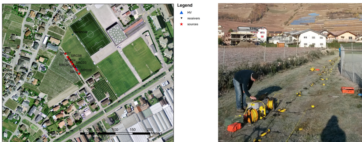
Figure 5: Left: overview map of the active seismic survey. ©2019 swisstopo (JD100042) Right: photo of the deployment.
