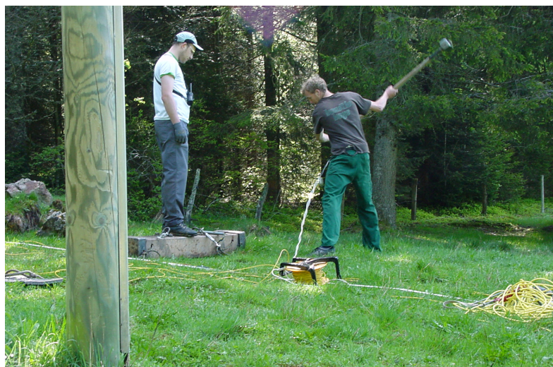
Fig. 2.1: S-wave data acquisition at profile 09SN_06BRANT-S1.
