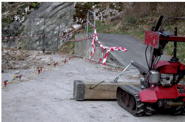
Fig. 2.1: S-wave data acquisition at profile 09SN\_02AIGLE-S1. In front: motorized barrow with shear wave source. In red the 4.5 Hz vertical receivers and in yellow the 10 Hz horizontal receiver. In background: portal into the military bunker.
