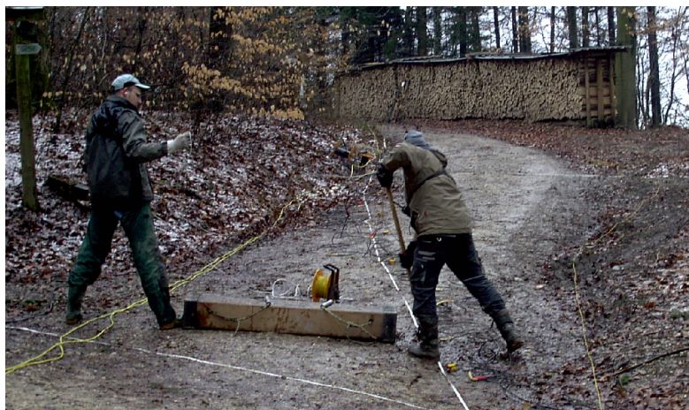
Fig. 2.1: S-wave data acquisition at profile 09SN_01ACB-S2.
